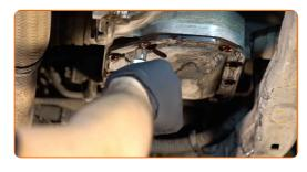
10 Remove the transmission fluid pan.
